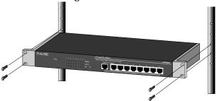
Figure 2-7 Mounting the FS4008DS in an equipment rack
